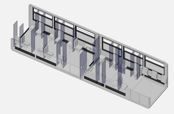
Using the pressure difference, on one side air inlets were created at the bottom and on the other side larger outlets causing this pressure difference, forcing the air to circulate inside the environment.
